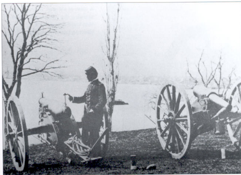
A 6-pdr. Wiard rifle. The novel gun with its special carriage is seen from both sides. (Library of Congress)
